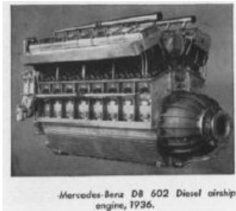
Figure 3: Mercedes diesel airship engine, 1936
