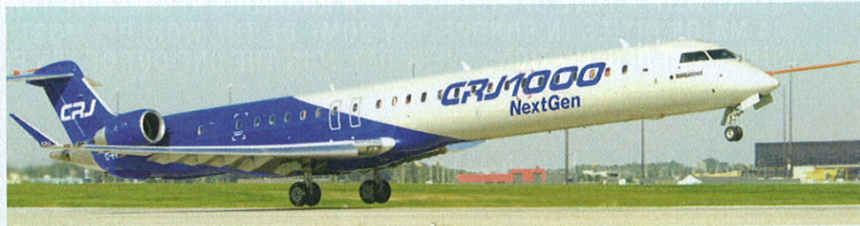
The 100-seater reached an altitude of 30,000ft and a maximum speed of 260kt
