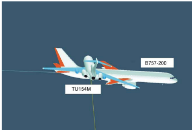
Reconstruction of the collision according to FDR data and collision evidence source: German Federal Bureau of Aircraft Investigations (BFU report 2004)
